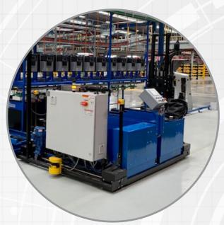
Every MAC system has a built-in emergency override & quick access stop button to support safe work practices and only requires servicing every 300 hours. The MAC battery handling equipment is perfect for operations needing medium volume fully automatic battery changing.
