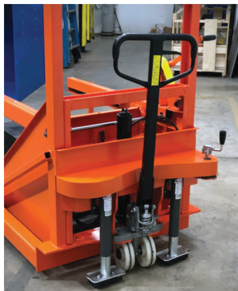
Optional hand crank activated positive braking system with no pushback when the brake is engaged
