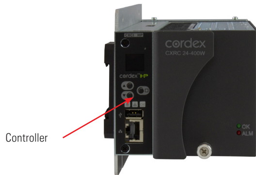
Figure 3: Cordex® CXCi HP system controller (integrated)
