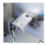
Hold the SPI in place using channel lock pliers while tightening nut. Torque to 130 in/lbs.
