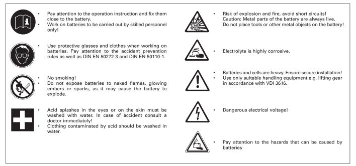
Ignoring the operation instructions, repair with non-original parts or using additives for the electrolyte will render the warranty void. For batteries according to the ATEX directive 94/9 EC, the instructions for maintaining the appropriate protection class during operation must be complied with (see relevant certificate).
