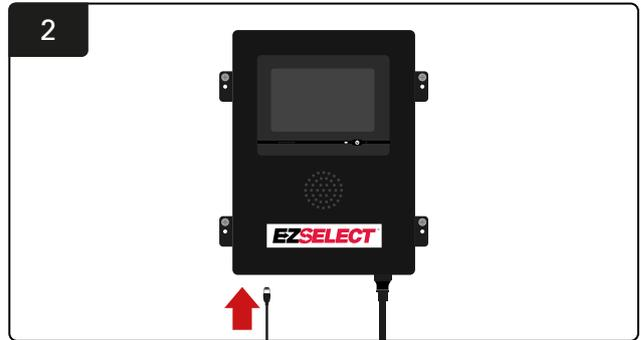
Insert the first CMD data cable into one of the available bus sockets on the Control Box.
